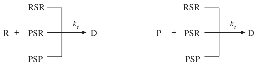
Scheme 2.12. Intermediate radical termination as the mechanism to explain the observed retardation in RAFT polymerizations. Initiating ( R ) and propagating radicals ( P ) terminate intermediate radicals RSR , RSP (adduct 2 , Scheme 2.8) and PSP (adduct 4 , Scheme 2.8). These reactions are added to the simulation comprising the radicals shown in Scheme 2.11.
